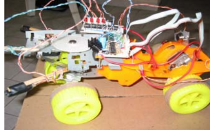
Figure 5. Mobile Robot of Ackerman configuration based on the PIC-PIC16F84.
